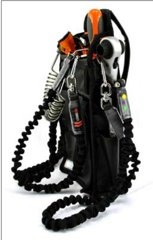
Advanced Linesmen's bag fitting system (secured around back-pad)
