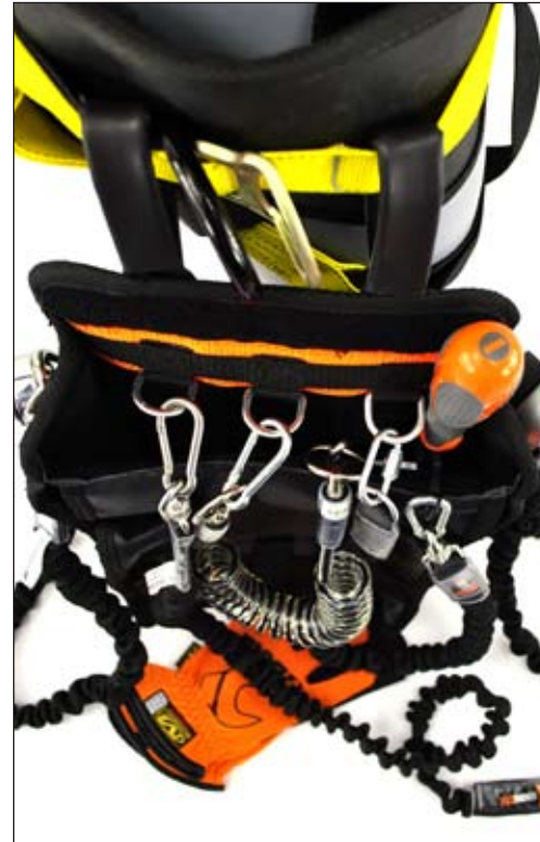
Advanced Linesmen's bag fitting system (secured around webbing belt strap)
